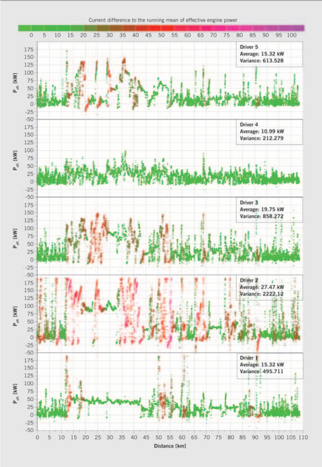
❷ Current variation of the moving mean about 60 s of the effective brake power, five drivers on FTA circuit
